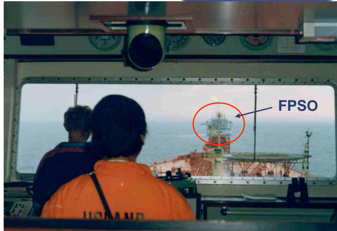
View from helmsman position – tanker aligned with FPSO
