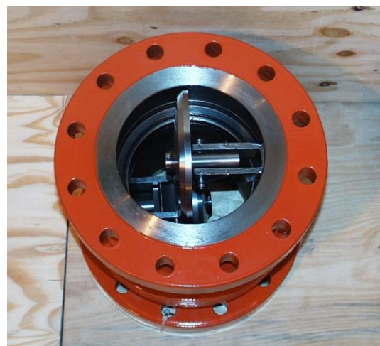
FIGURE 1 MBC WITH INTERNAL FLAP VALVE
