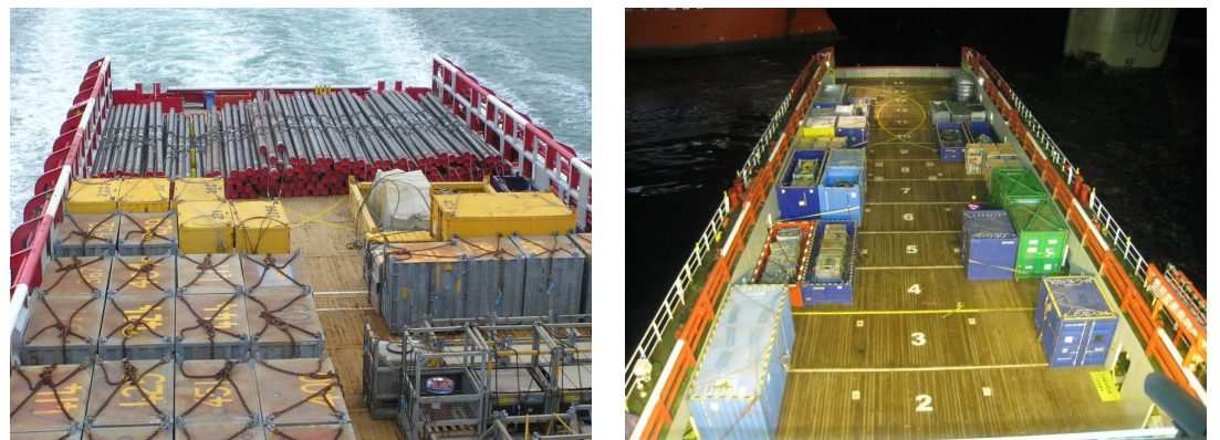
Figure 5.3: Block stow (in conjunction with cargo securing)
