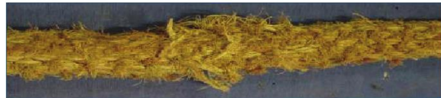
Figure D3: Damaged Rope
