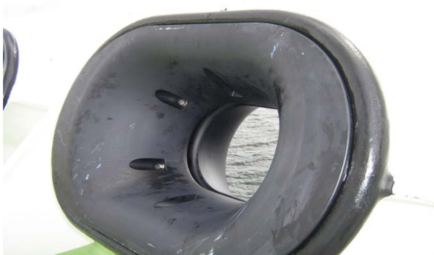
Figure 1.3: An example of a low-friction, low-abrasion fairlead insert
