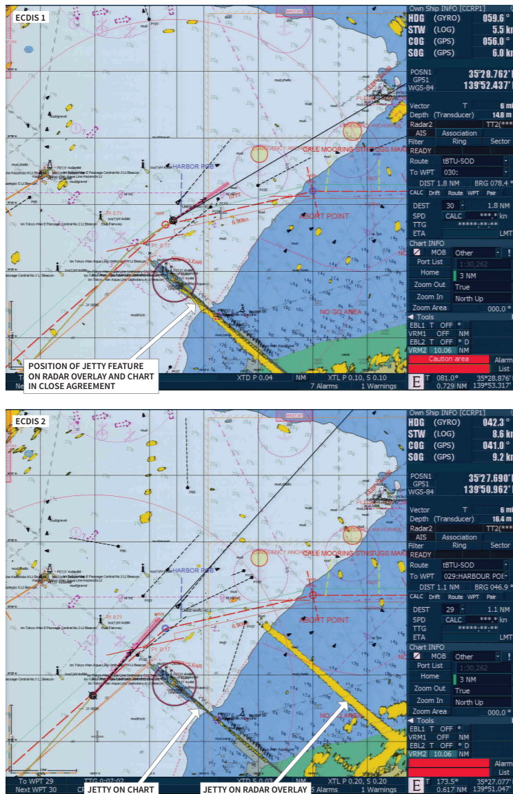
Figure 3: ECDIS screenshots illustrating radar overlay discrepancy
