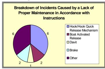
Problems with Hook/Hook Quick Release Mechanism top this grouping. Usually attributable to wastage critical of parts within safety mechanisms.
