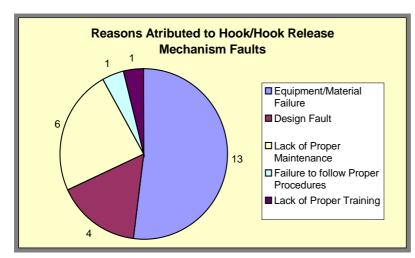
previously As incidents noted. attributed to faults with Hook/Hook release Mechanism are the greatest single group. Of these 25 incidents. over 50% are due to failure of the equipment or of the material. When
